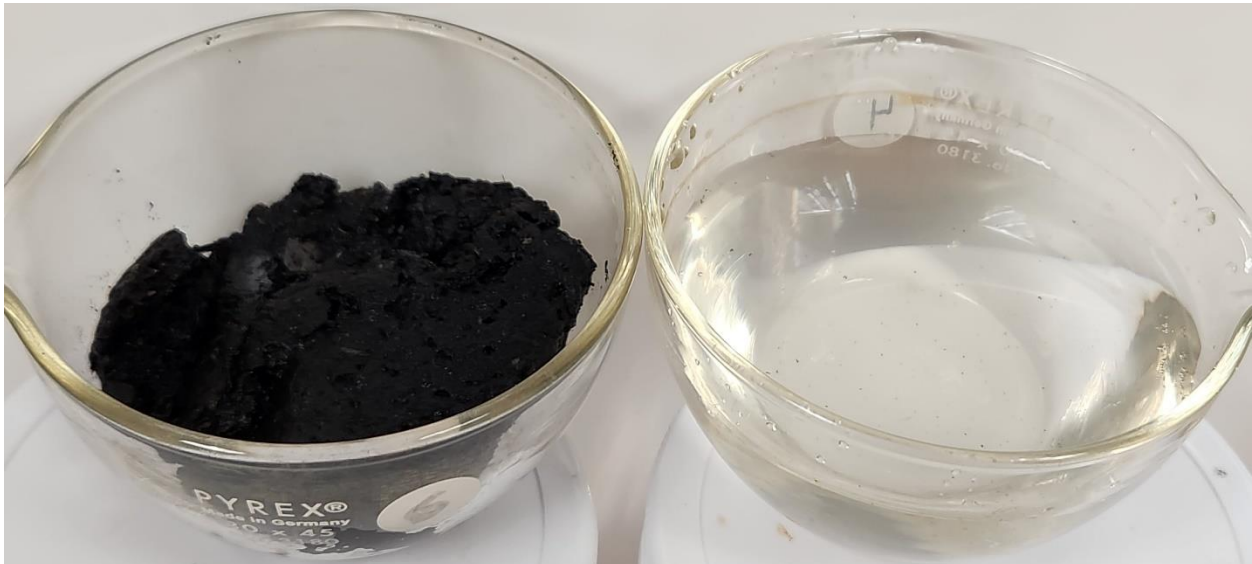
One thousand milliliters of diluted sample conditioned with Solve 9244 was poured through geotextile tube fabric, the dewatered cake (left) and captured filtrate (right) are displayed above.
